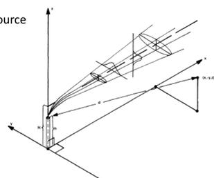
Figure 4. Cooling tower risks and sprinkler risks modeled according to a modified Gaussian plume model. An aerosol size distribution was simulated for both sprinklers and cooling towers.
