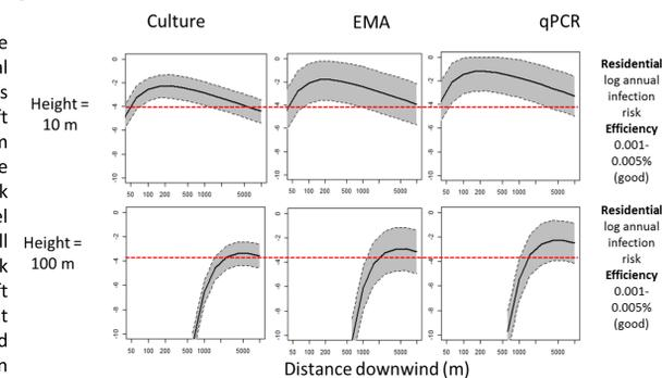
Figure 7. Cooling tower risk models shown for wind speed = 7 m/s and RH = 65% (most conservative scenario). Red lines are associated with the drinking water annual infection risk benchmark for reference ( $10^{-4}$ ).<sup>12</sup>
