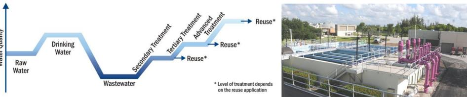
Figure 1. (left) Schematic for reclaimed water treatment; and (right) Example of reclaimed water system from Boca Raton, Florida<sup>3</sup>
